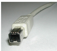
Thermal Digiplate side is a type B connector(square)
